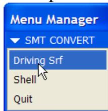
Select “Driving surface” from the menu manager and select inside surface of first cone. Give a wall thickness of 1 mm (this will be the actual sheet metal part thickness.).
