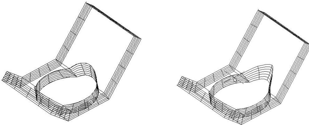
Figuur 4: surface model of a bracket.
